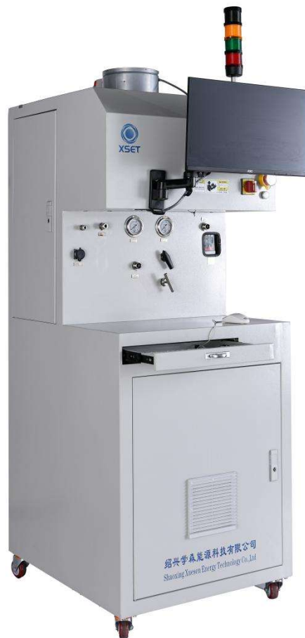
Fig.7 Picture of hydrogen circulation system test bench
